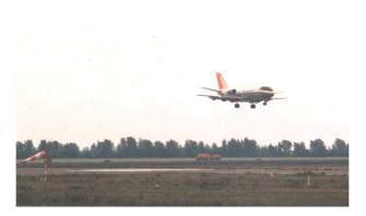
DLR's aircraft ATTAS, conducting an automatic landing using control laws that include Dymolagenerated inverse model code as its kernel.
